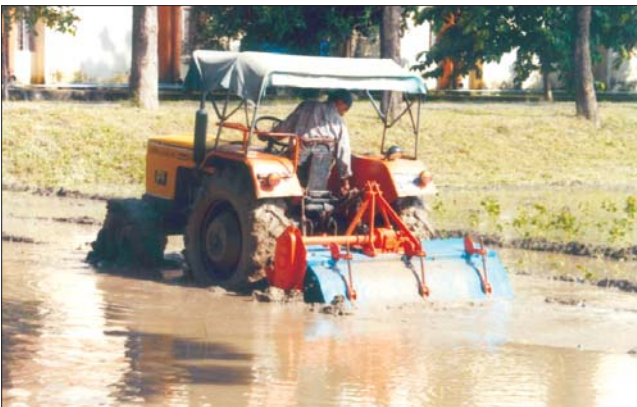
Tractor-operated lug wheel puddler for high speed shallow puddling of rice fields
