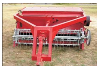
Modified cutter-bar type rice-straw chopper-cum-spreader
