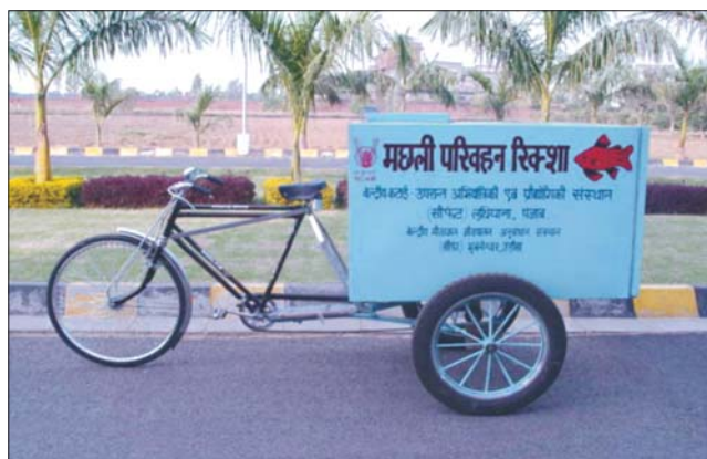
Mobile cool chamber with a conventional cycle rickshaw for short distance transportation of fish
