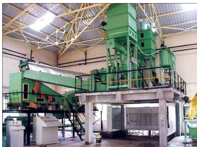
Pilot plant to manufacture particle boards from cotton plant stalks
