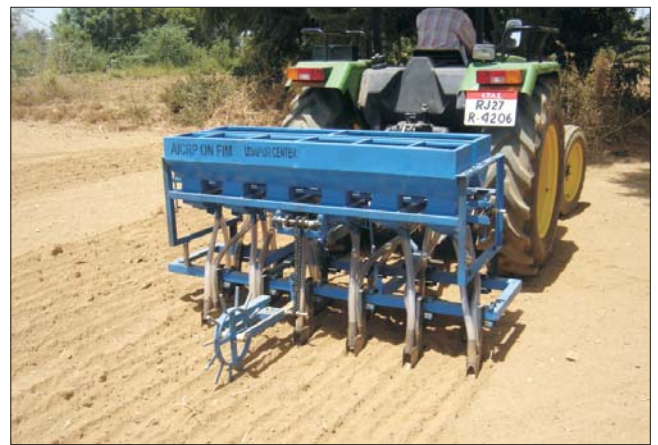
Tractor-mounted garlic planter. The observed seed rate during testing varied from 500 to 700 kg/ha depending on size of garlic cloves
