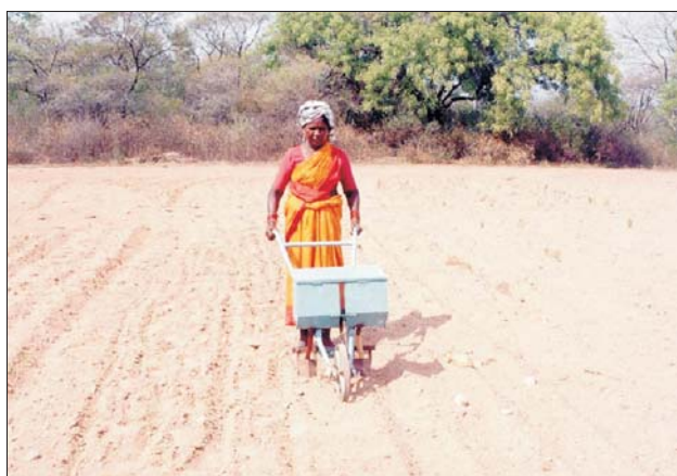
Hand-drawn seed drill. This two-row seeder developed with suitable attachments can be used as a seed drill or as a weeder
