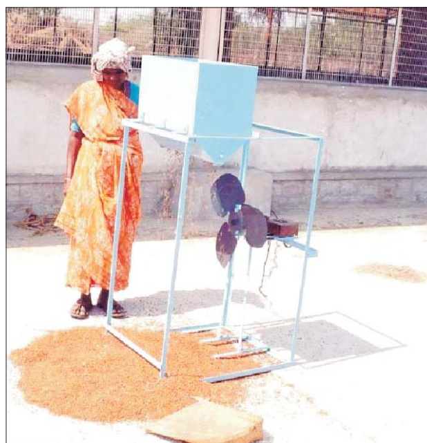
Hand-operated winnower. For this machine, 2 women are required and they can winnow 0.25–0.3 tonne of grains per hour
