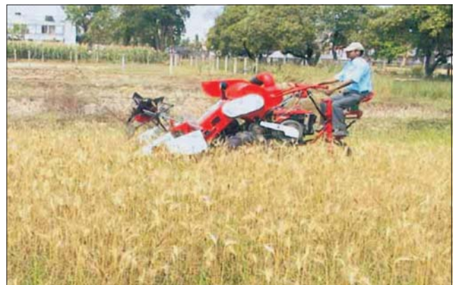
The field performance of mini combine was assessed for wheat crop at moisture content of 15.4% (db)
