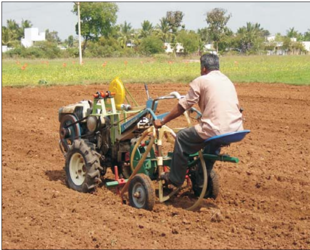
Power tiller-mounted air-assisted seed drill for sowing small seeds like sesame, cumbu and sorghum
