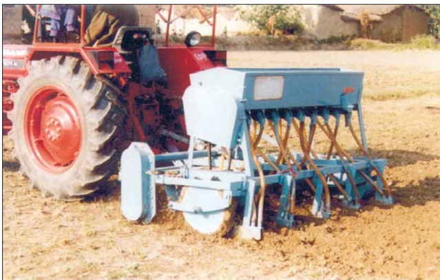
Zero-till seed-cum-fertilizer drill in operation. The machine was demonstrated at Pantnagar (176 ha) and Jabalpur (650 ha) at farmers' field
