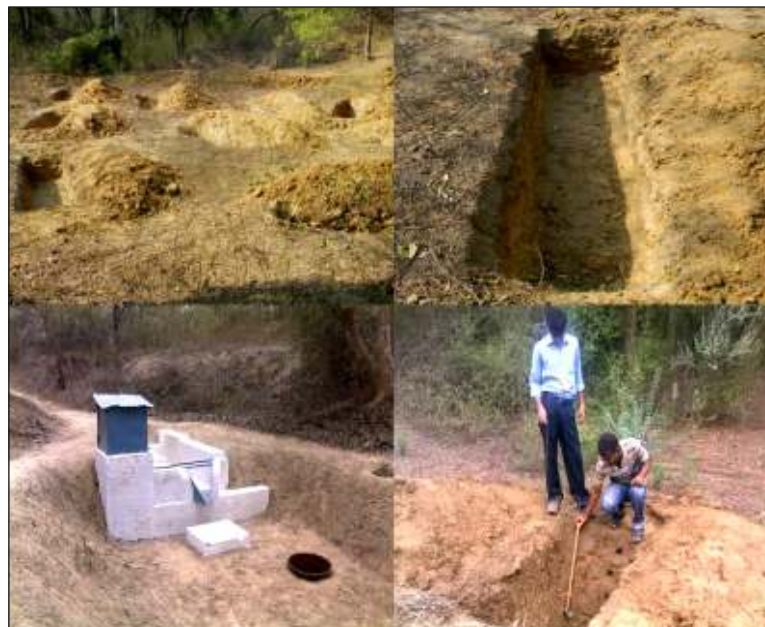
Photo 4.1 : Trench lay out, renovated gauging structures and soil profile studies at watersheds
