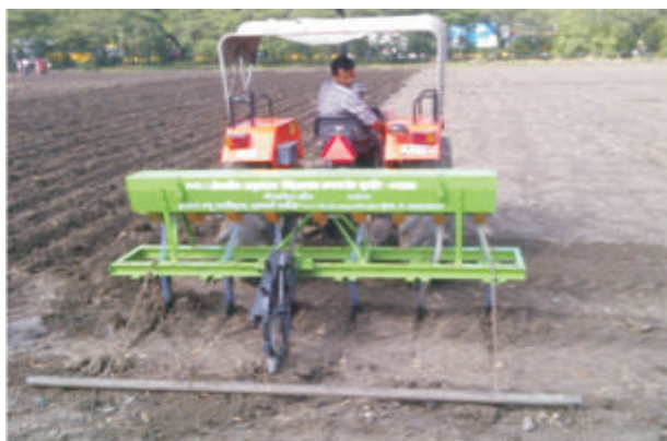
Fig. 24. Two in one (Soybean seed drill cum planter)
