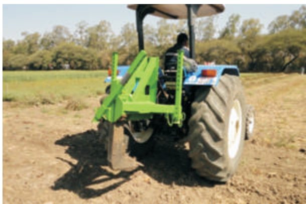
Fig. 22. Sub soiler developed at DSR, Indore
