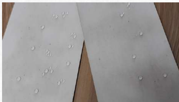
Figure 2. Hydrophobicity of sugarcane wax coated paper.
