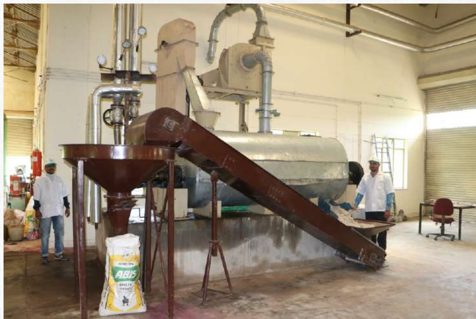
Figure: Different components of the designed and modelled Rotary Tubular Drum Dryer (top) and the Rotary Tubular Drum Dryer
