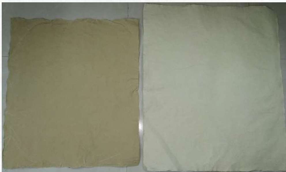
Figure 3. Pulp sheet prepared from banana fibre and cotton: banana (90:10) blend
