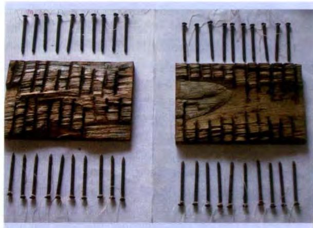
Nails retrieved after corrosion studies
