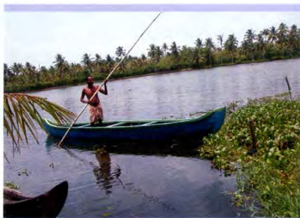
An FRP sheathed rubber wood canoe after three years of operation
