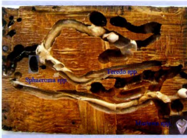
Untreated rubber wood panel after exposure for 12 months in the estuarine condition
