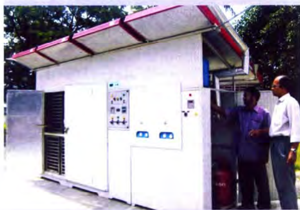
Solar dryer with LPG back up
