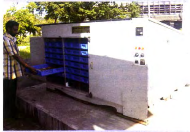
Fish dryer using renewable energy, supported with electrical heating system
