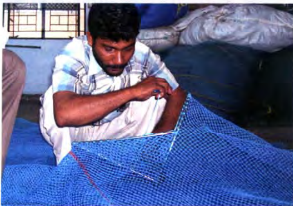
Fixing of Fish eye BRD to the shrimp trawl codend
