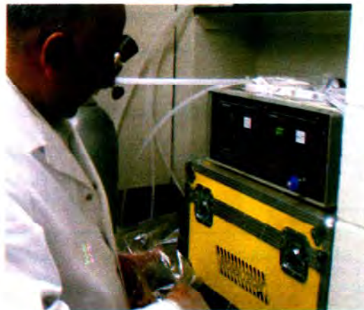
Dr. T.K. Srinivasa Gopal measuring the headspace gas in MAP salmon samples using MOCON Oxygen and Carbon dioxide analyser
