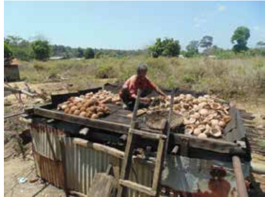
The broken coconut is arranged on the stage and burned from below using coconut wastes
