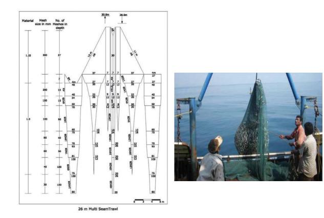
The 26 m multi seam trawl is fabricated with 14 seamswith seven panels. The seams are strengthened by supporting ropes. The mouth of the trawl is made with large mesh and the body netting is graduated as it narrows with decreasing mesh sizes of the lighter ranges of nylon twines. System consists of an 18 m four panel semi-pelagic trawl with double bridles, front weights of 25 kg each and vertically cambered high aspect ratio otter boards (trawl doors) of 85 kg each.
