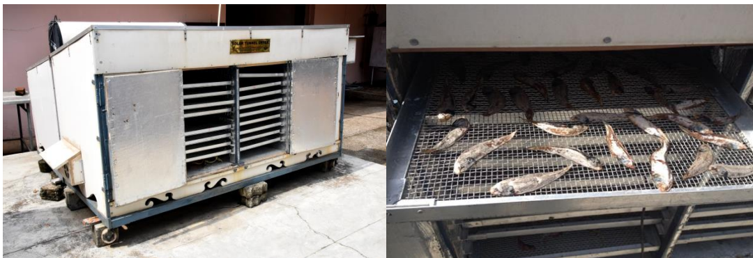
Fig.5. CIFT Solar-Cabinet Dryer with Electrical back-up
