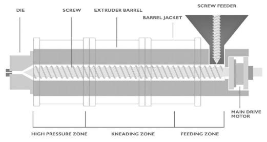
Pre-conditioning is not applied to all extrusion processes. It is applied when moisture contents around 20 to 30% and long residence times are required for of the material. Pre-conditioning favours uniform particle hydration, reduces retention times within the extruder and increases throughput and increasing the life of the equipment, due to a reduction in the wearing of barrel and screw components. It also reduces the cost of energy involved in the process.
