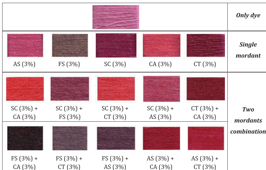
FIGURE 2 Colors obtained from dyeing of woolen yarn with cochineal extract in presence of mordants in single and combination form.
