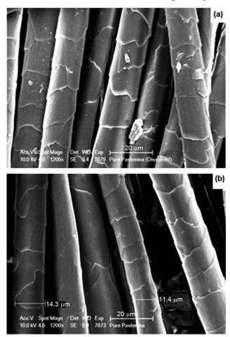
Fig. 1—SEM images of machine-spun (a), and hand-spun (b) pashmina yarns
