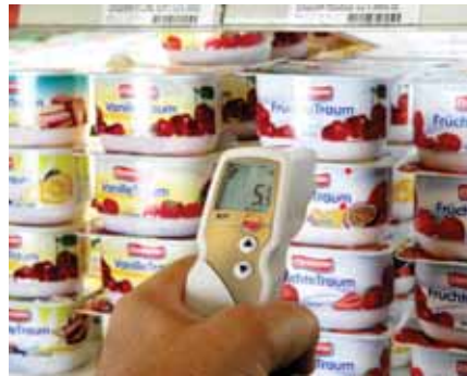
Measurement in refrigerated shelving with testo 831
