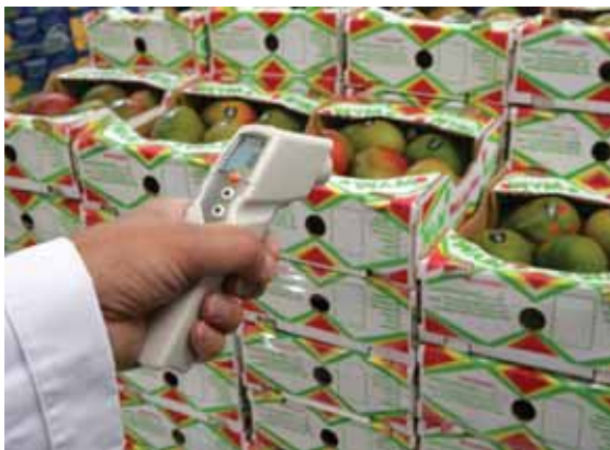
Checking temperature in Incoming Goods with testo 831
