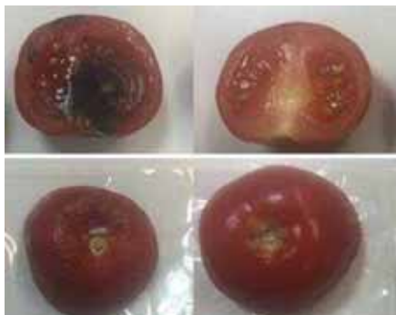
Control tomatoes (left) rotted after six days while those wrapped in a new clay-based film (right) stayed fresh. Photo: Hayriye Ünal
