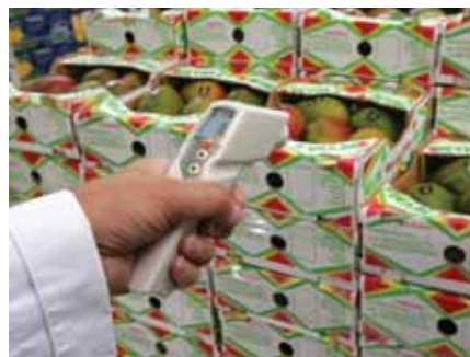
Measurement in refrigerated display with testo 174
