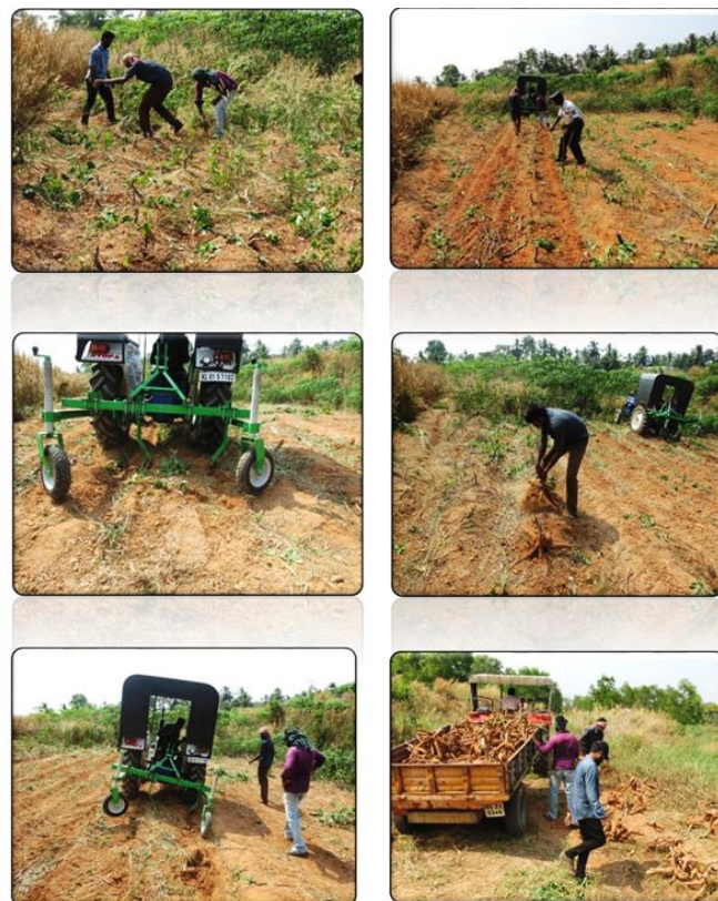
Fig 3: Harvesting trials with single row TNAU cassava harvester
