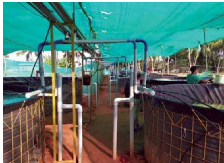
Flow-through based Seabass Nursery System
