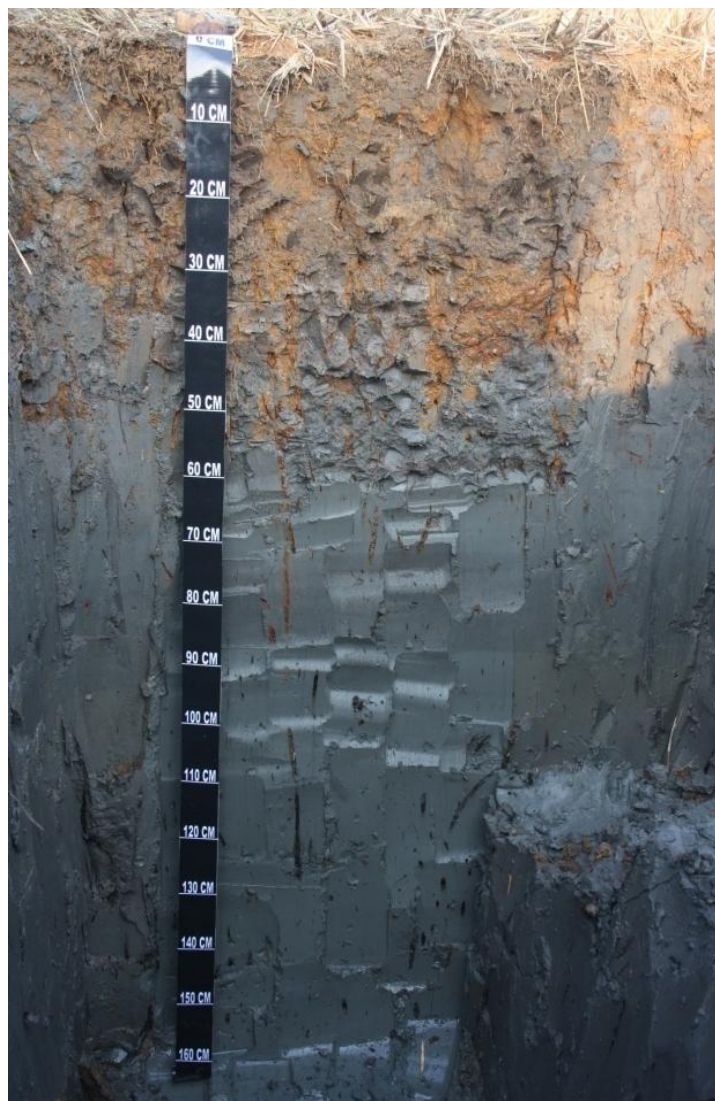
Figure 2: Soil profile of Kuttanad Kayal (Acid sulphate soils): Salidic Sulfaquepts (Source: NBSSLUP Archives)
