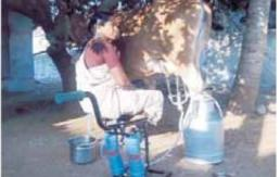
A view of hand operated single cow milking machine (Valarpirai Milker) and milking by using it
