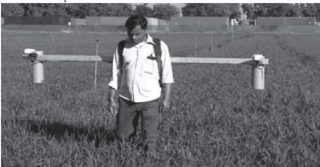
Fig. 1 NDVI based variable rate urea applicator for rice and wheat crop
