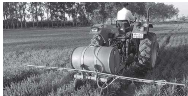
Fig. 2 Sensor based real-time uniform rate spraying system
