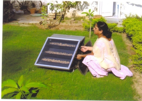
Multi-rack solar dryer
