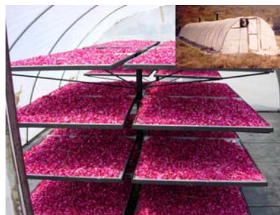
Rose petal drying in solar tunnel dryer
