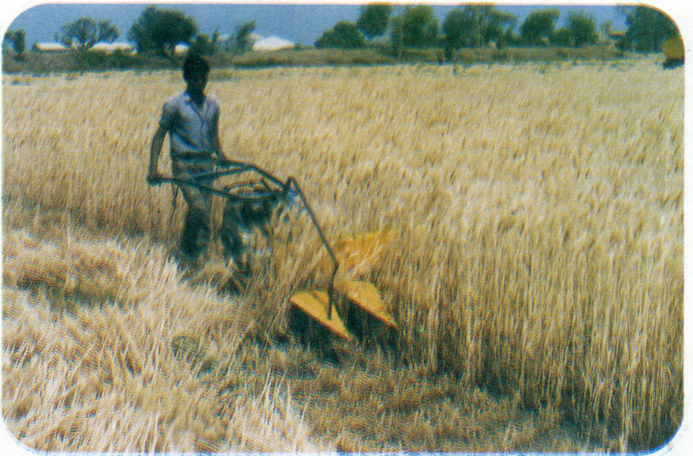
Fig. 6. Wheat harvesting by vertical conveyer reaper (Self-propelled)
