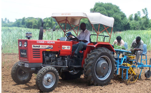
Fig. 6 Field operation of two row tractor drawn mechanical planter for sugarcane bud chip settlings raised in protray (side view)
