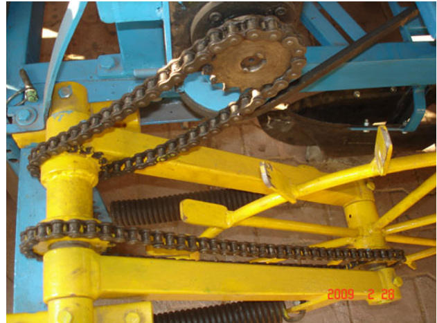
Fig. 2 Power transmission mechanism in sugarcane bud chip settling planter
