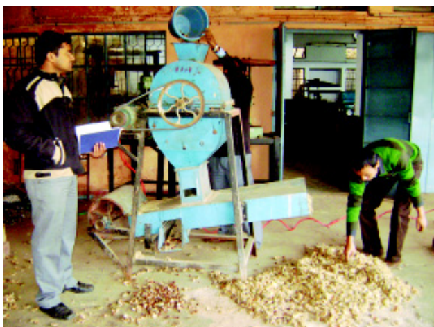
Fig 1 Test run of arecanut sheller
