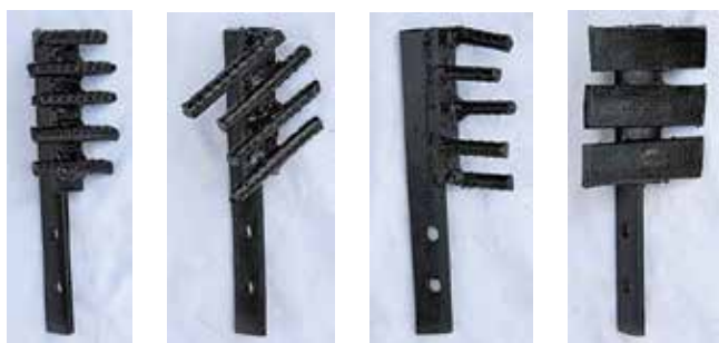
Rod parallel to the shaft Rod 45° to the shaft Rod perpendicular to the shaft Flat parallel to the shaft
