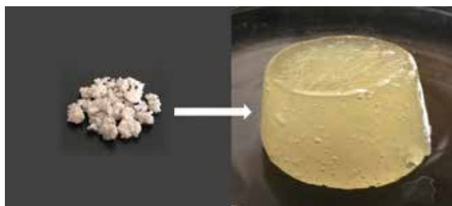
Fig. 51: Cross-linked guar gum hydrogels (dried and swollen stage)
