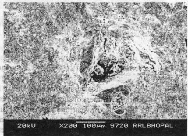
Microstructure at 0.47A (Cracks are visible at high peening intensity)
