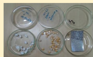
Synthesized nano- fibre matrix (10 % PVA + 100 ppm GA 3 )
