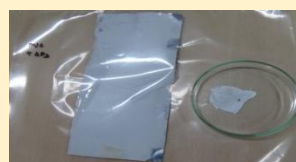
Synthesized nano- fibre matrix (10 % PVA + 100 ppm GA 3 )
