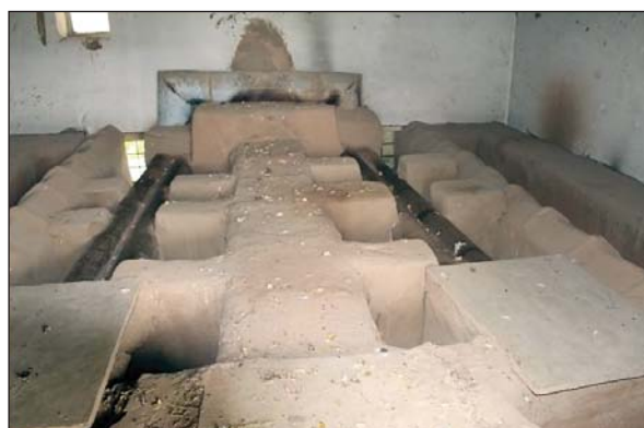
Mud wall duct for curing
