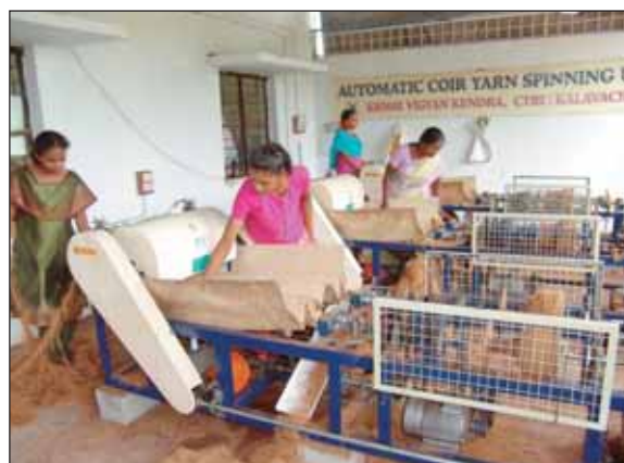
Training in Coir 2-ply yarn making on automatic machine
