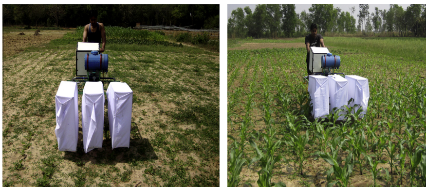
Fig. 6. Performance evaluation of herbicide applicator in maize and groundnut field.
