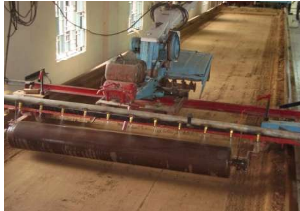
Fig. 5: Soil bin preparation for experimentation
