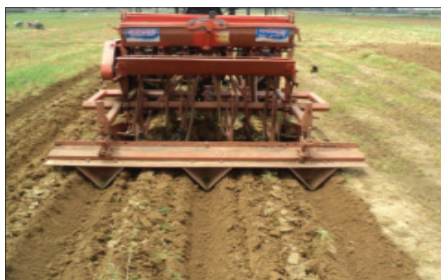
Plate 2.8.5. Sowing of crop on permanent broad bed seed cum fertilizer drill and furrow irrigation
