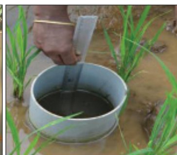
Plate 4.3.3. DPW measurement inside the field water tube during irrigation
