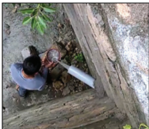
Fig 3.1.2. Observation of flow rate through filter
