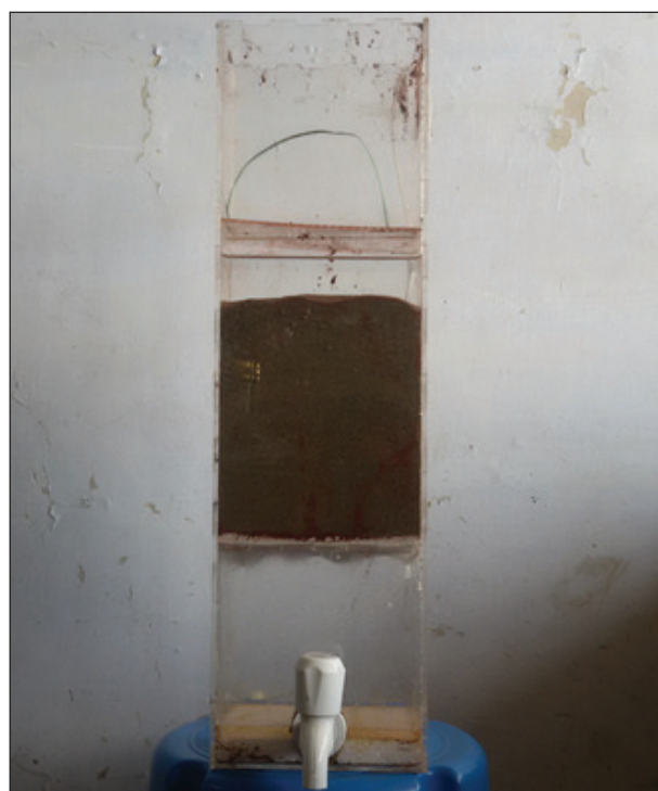
Fig. 4.2.7(b). Uncoated sand filled in material container
