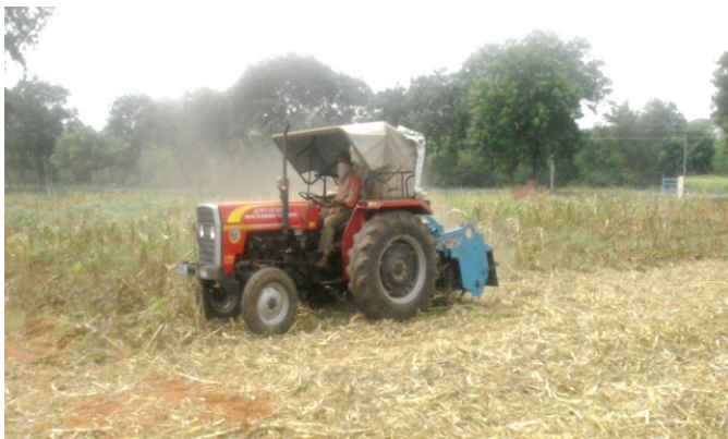
Solid model and operating prototype of crop stalk shredder
