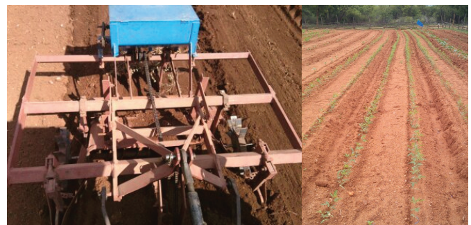
Tractor drawn Raised/permanent bed planter Red gram crop on raised beds
