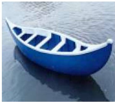
Fig 9. FRP-Coated Rubber Wood Canoe
