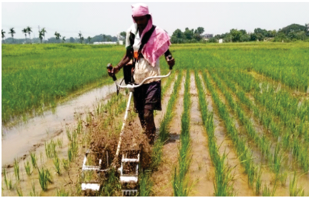
Mechanical weed control by power weeder
