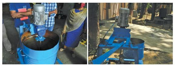
Custom soil puddling machine using 0.5 hp electrical motor
