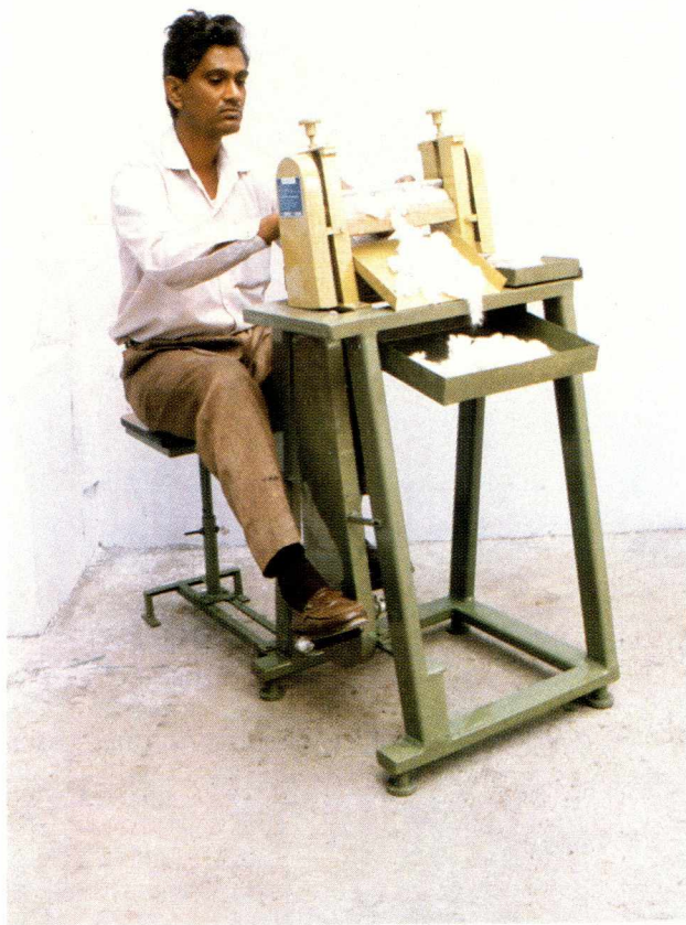
Foot-operated Kisan Gin designed at CIRCOT
