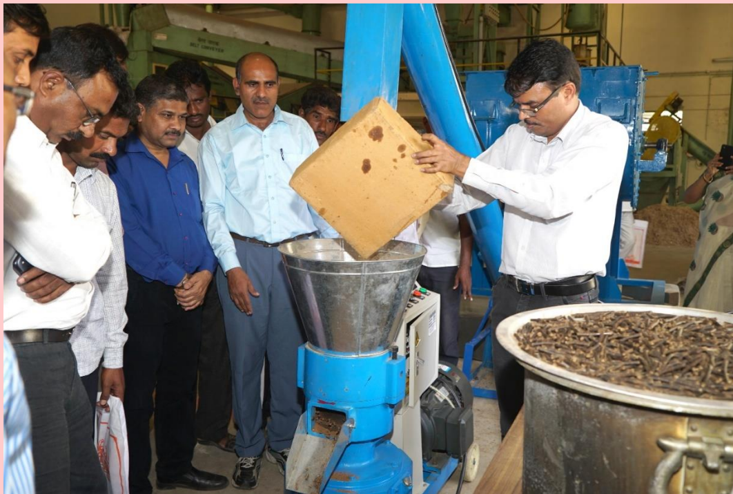
Demonstration of pelleting of cotton stalks to the farmers and stakeholders at GTC, Nagpur
