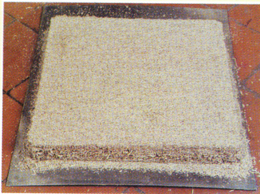
Three layered mat of different particles
