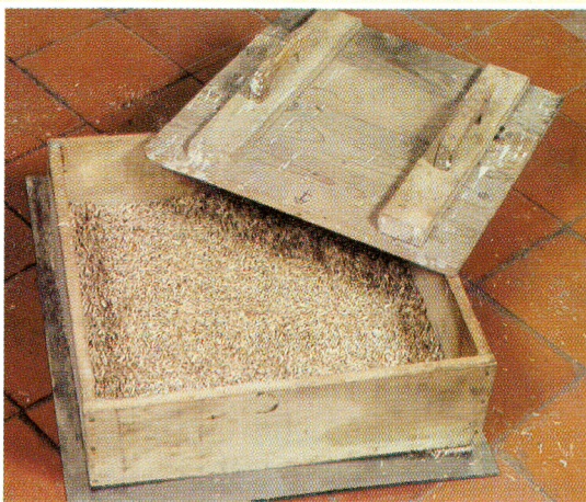
Mat formation of particles coated with resin
