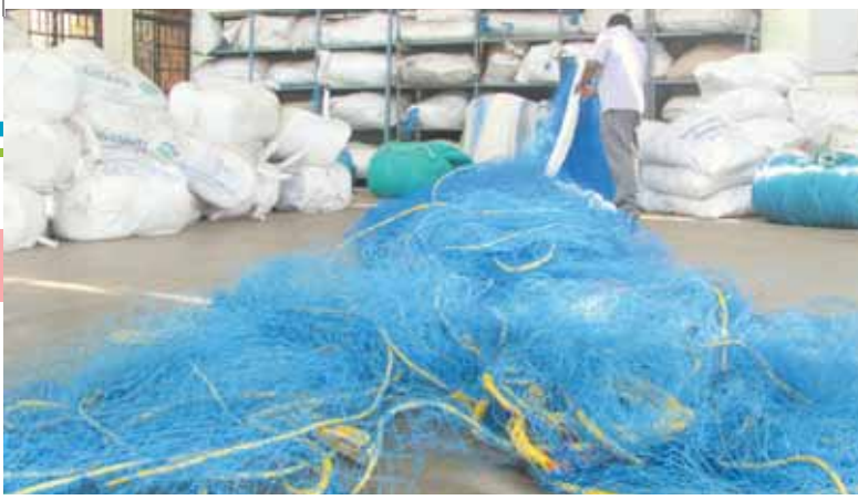
Fabrication of 23.5m myctophid trawl
