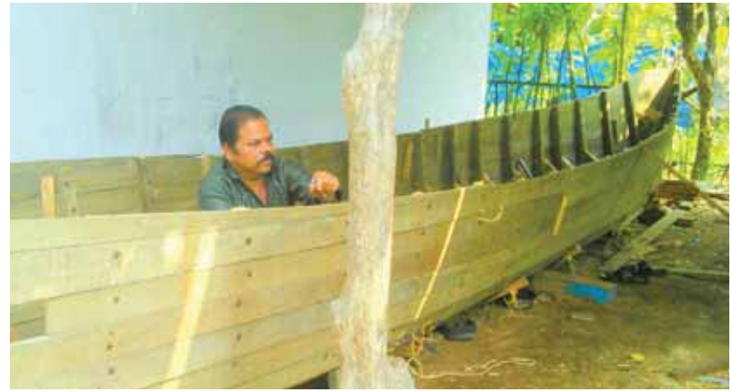
Coconut wood canoe under construction
