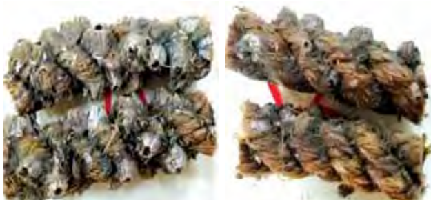
Manila rope exposed to marine environment for 30 days
