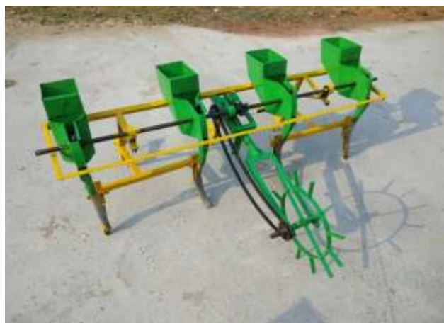
Fig. 2.11 Urea briquette applicator attachment for self-propelled rice transplanter
