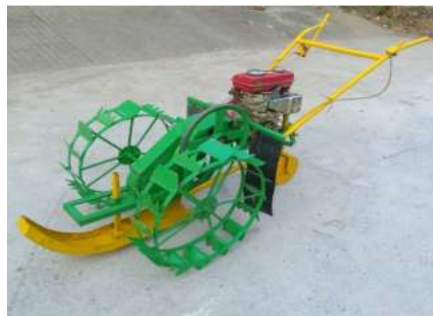
Fig. 2.12 Power operated two row wet land weeder for rice
