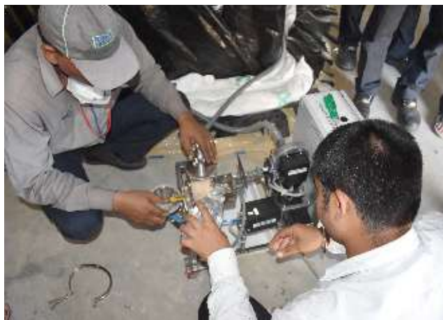
Fig. 3.31. Initial preparations with PH 3 gas generator
