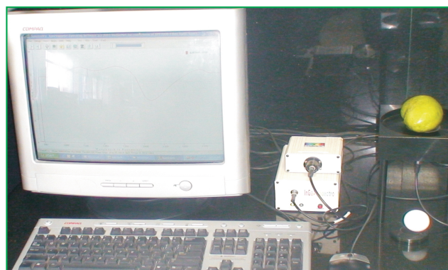
Fig.2. Fibre optic spectrometer in operation for spectra acquisition using developed sample holder
