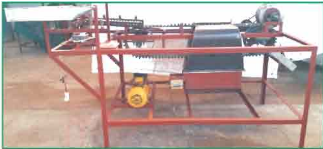
Fig 3. Prototype of Chilli destalking machine
