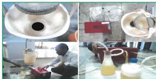
Fig 43. Set-up of carbon filter and vacuum filtration of kinnow juice
