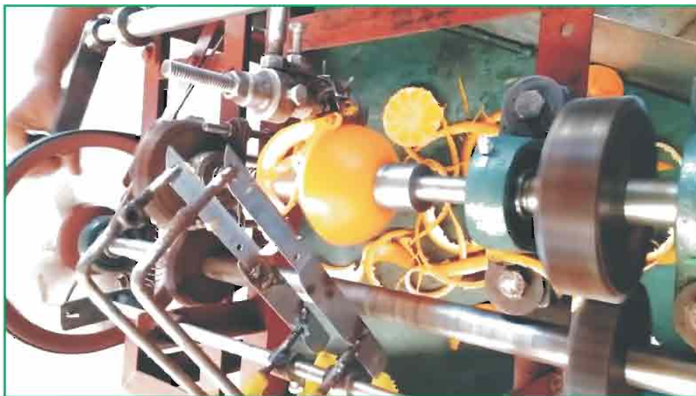
Fig 4(b) Semi-automatic peeler for sweet orange and kinnow
