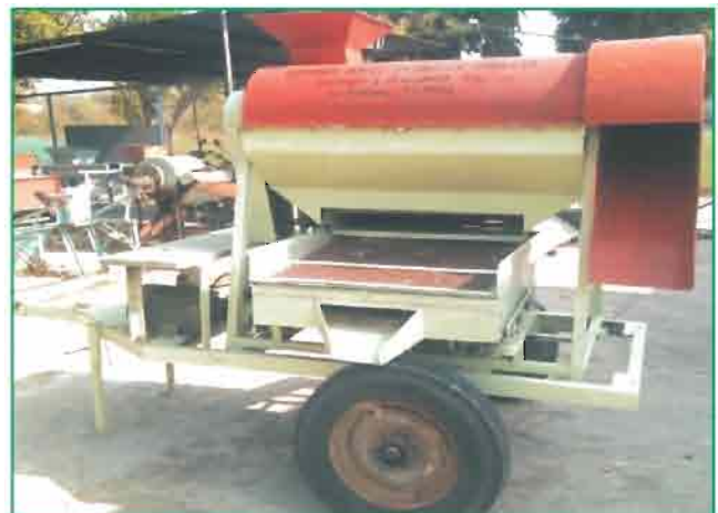
Fig 64. Improved maize dehusker-cum-sheller
