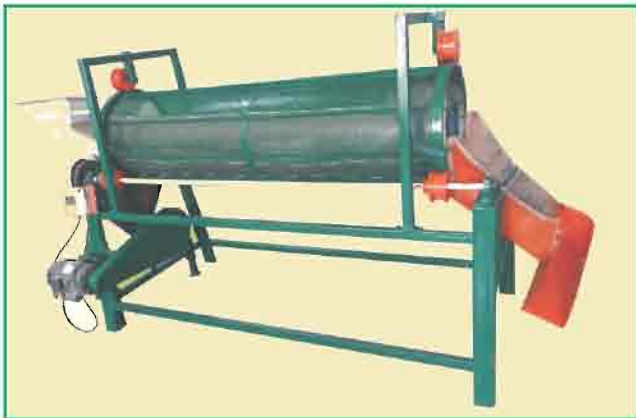
Fig 71. Continuous sapota cleaner (Capacity 550 kg/h)
