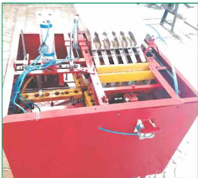
Fig 1-Pneumatic assisted coring device
