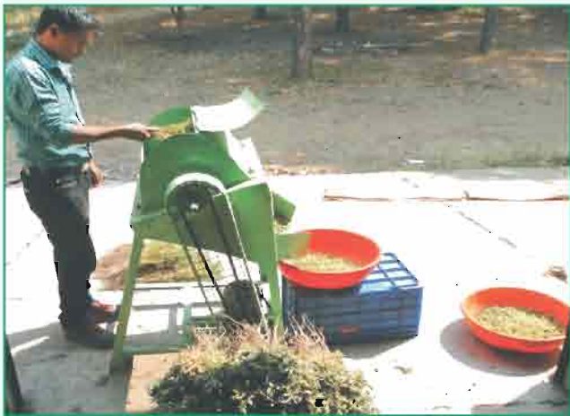
Fig 62. Green chickpea pod stripping machine
