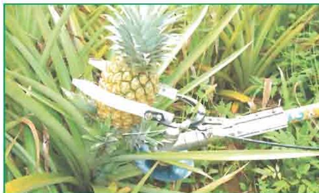
Fig 67. Manually operated pineapple harvester
