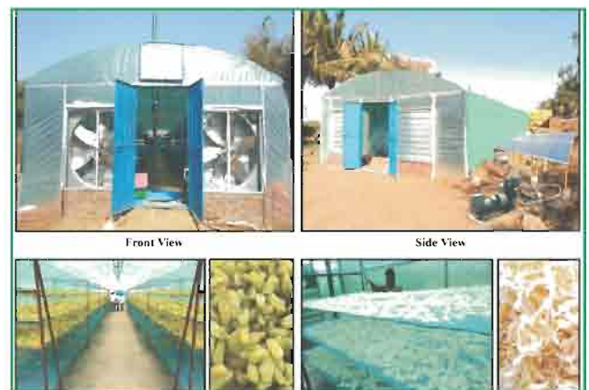
Fig 72. Multi-mode solar dryer
