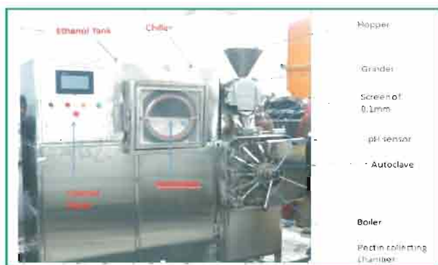
Fig 66. Pilot plant for pectin extraction
