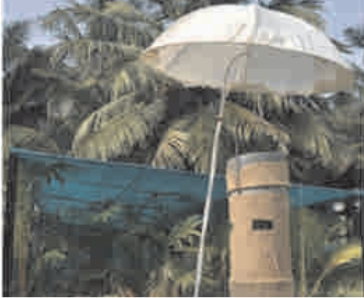
Fig.21. Umbrella studded redesigned PVC trap
