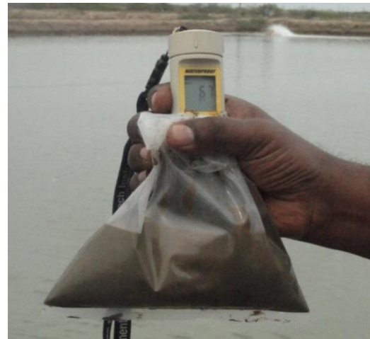
On-farm measurement of redox potential
