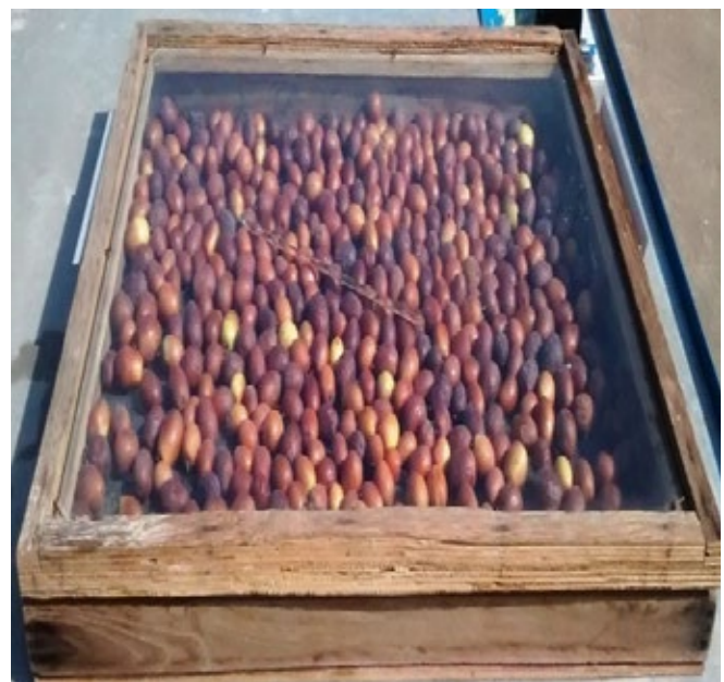
Fig.1: Solar dryer in Ziziphus mauritiana (ber) loaded condition
