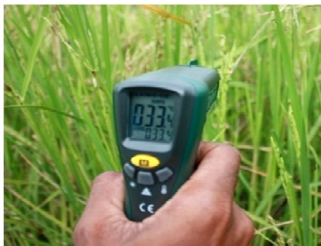
Fig. 12(d) : Panicle temperature measurement using Infrared Thermometer
