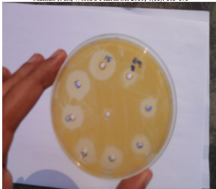
Fig. 3b: Determination of MIC of ethanolic extract of A. nilotica gum for a Staphylococcus aureus strain (MIC of the strain was 100 µg), the centre well is control negative filled with only DMSO while periphery wells contain the extract in DMSO (50 µl) [Anti clock wise 5 mg, 2.5 mg, 1.25 mg, 640 µg, 500 µg, 400 µg, 200, 100 µg]
