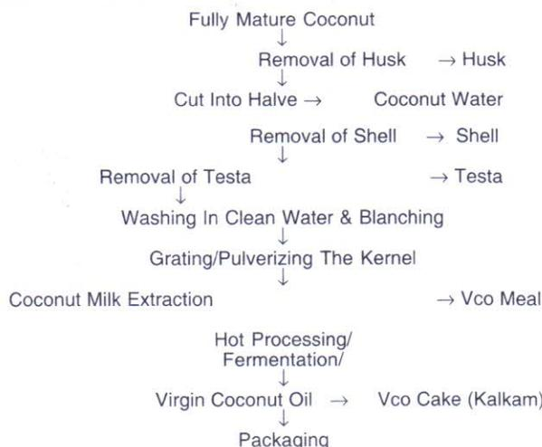
Fig. 1 : Process flow chart for the production of virgin coconut oil
