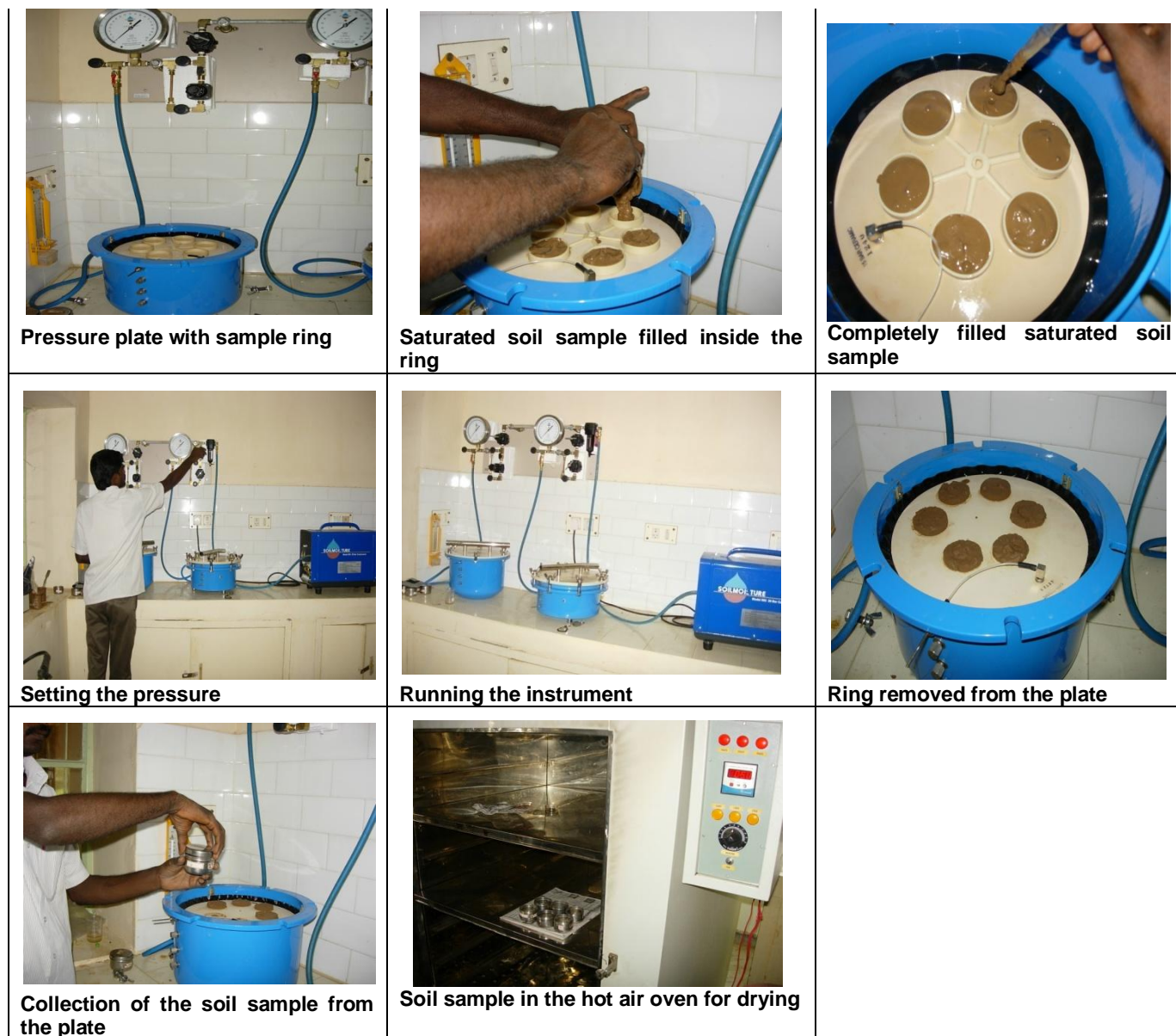
Figure 1. Soil moisture measurement by using pressure plate membrane apparatus.
