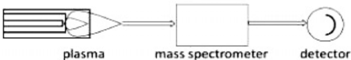
Fig. 3. Working principal of inductively coupled plasma mass spectrometers
